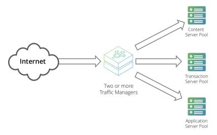
You can install two or more Traffic Managers in a clustered configuration to provide full fault-tolerance for individual software failures. A typical configuration contains at least two Traffic Managers, and at least two servers hosting the load-balanced application.
