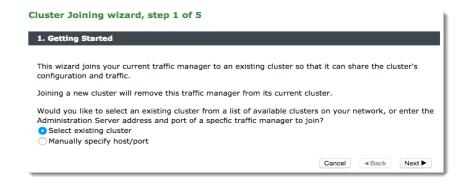
To instruct the Traffic Manager to automatically scan the network for contactable Traffic Managers, click "Select existing cluster". Alternatively, to enter a specific hostname and port you want to join, click "Manually specify host/port".
