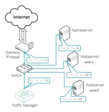
By installing a Traffic Manager, configured to receive traffic over a single network port and IP address xx.xx.xx.3, you can alter your DNS record to instead direct clients to xx.xx.xx.3. In this way, the Traffic Manager receives the Web page requests and responds with content from one of the available Web servers.
