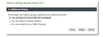
To add the Traffic Manager to existing Traffic IP groups, click "Yes, and allow it to host Traffic IPs immediately". However, this can result in a number of connections being dropped at the instant the new Traffic Manager is added to the Traffic IP group, because allocations of traffic need to be transferred to the new Traffic Manager.
