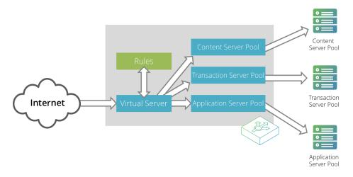
A pool is a collection of nodes. Each node corresponds to a back-end server and port, such as server1.mysite.com:80. You can set up several pools with nodes in common.
